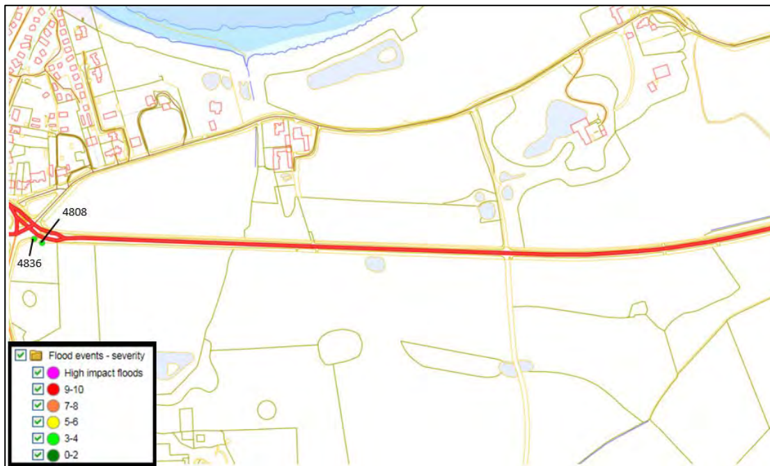
Figure 2-10: HADDMS Recorded Flood Incidents between Garstang Road and the approach to Windy Harbour Junction (not to scale)
